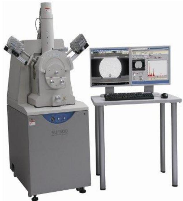
Figure-1: Overview of the SEM/EDS Unit
